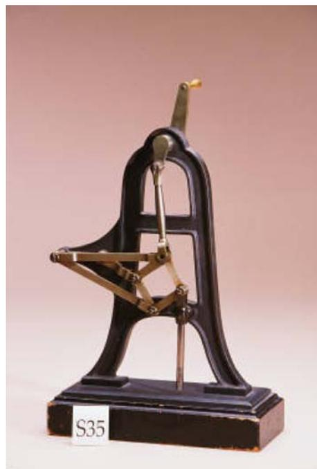
**Fig. 2** Peaucellier straight line mechanism (<http://KMODDL.library.cornell.edu>)
