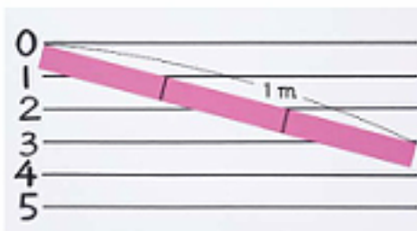
How to Divide a 1 m Tape into 3 Equal Parts
