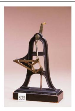
Fig. 2 Peaucellier straight line mechanism (http://KMODDL.library.cornell.edu)
