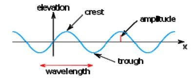
Usually a tsunami has a main crest whose height h was not much more than a metre. The wavelength L would have been roughly of the order 300 km. So the maximum slope of the surface would have been roughly  $2\pi h/L$  - only about 1 in 50,000. Such a tiny slope would be quite invisible from any of our vantage points.
